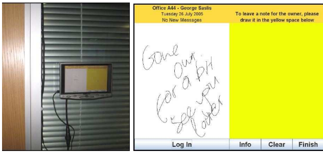
Figure 2: Hermes II doorplate display deployed outside an office with the messaging interface shown on it.
