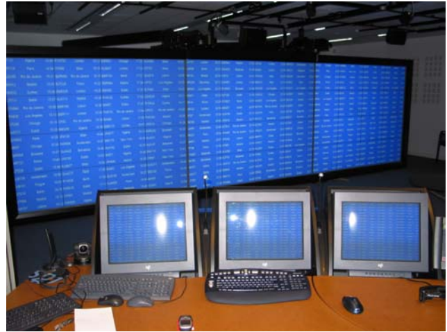
Figure 6. Display set-up, using a 3-screen CADWall to simulate the physical characteristics of a very large information display comprising details of 240 flight departures.
